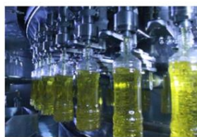
ITO EN has developed a proprietary room-temperature aseptic filling method that does not require the use of germicides in sterilizing bottles.
