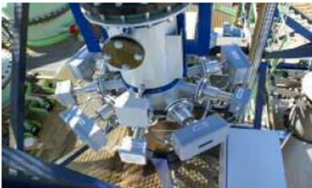
Laser-type gas concentration measurement equipment
