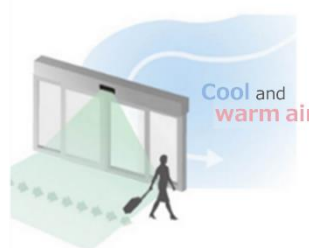
e-Smooth Sensor monitors the direction of people walking to reduce the unnecessary opening operations for automatic doors
