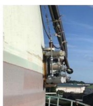
Scene of work with a machine Removal of the paint by a skilled worker using a blasting method
