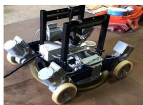
Shot-blasting machine Spherical gas holder (the upper hemisphere shot-blasted)
