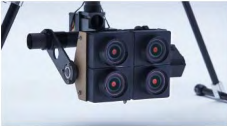
4-eye high-speed camera for measurement surveying
