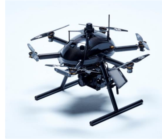
Left : Smokestack inspection drone (ACSL – PF2)
