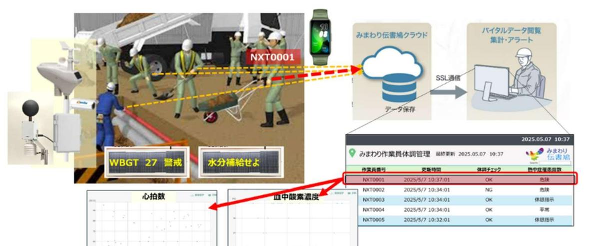
The diagram illustrates the system's workflow: data from the construction site (including WBGT 27 and heart rate) is sent via SSL to a cloud for storage and then to a server for processing. The processed data is then displayed on a mobile app interface, which shows a table of worker health status and a graph of heart rate and blood lactic acid temperature.
