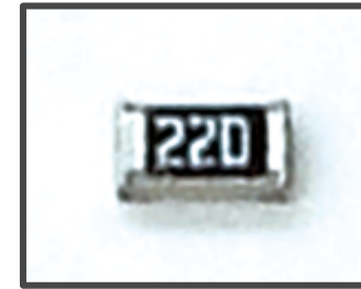
Letter/shape imaging (Small chip parts; about 1mm)
