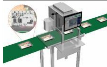
Inspection of use-by dates printed on packages
