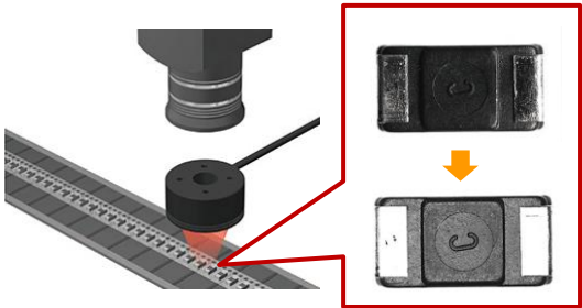
Visual inspection solution for electronic components
